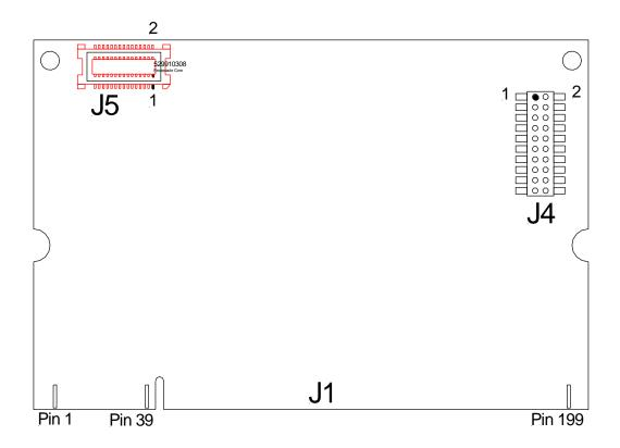
Red colored parts are located on the bottom side of the CPU module.
